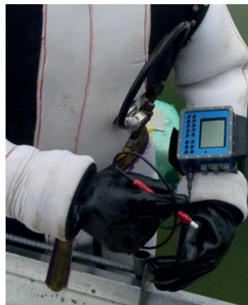
Fig. 5: The input unit is strapped to the diver's arm; the magnetic stylus allows the diver to operate the device and trigger measurements (photo: Zurich Underwater Archaeology Section, Department of Urban Development).
