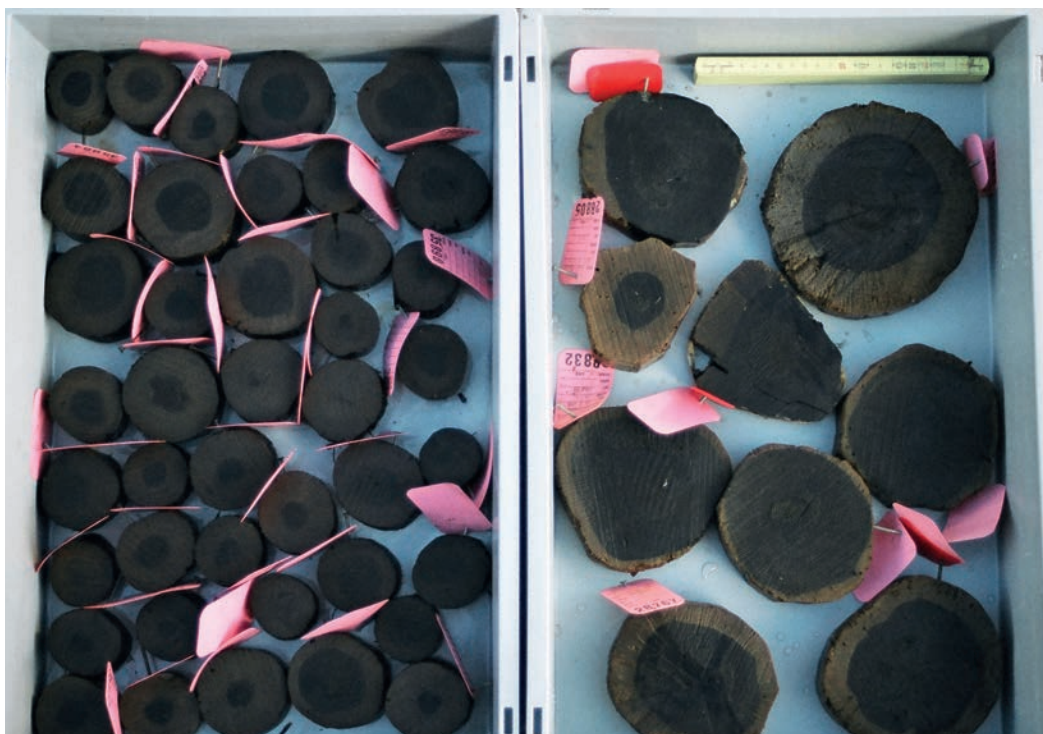
Fig. 5: Oak samples cut and prepared for dendrochronology. An approximately 3 cm slice is taken using a band saw. This equipment leaves the wood with a flat smooth-surface greatly aiding speed in sample preparation and saving razor blade costs (photo: John Francuz).
