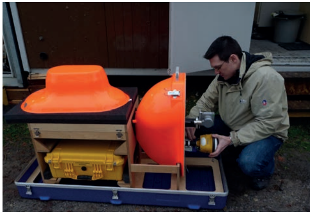
Fig. 3: Open transport case with Hydra and a case with accessory equipment (photo: Zurich Underwater Archaeology Section, Department of Urban Development).
